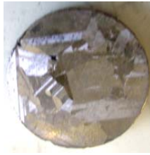
FIGURE 1. Optical photography of one of the polycrystalline GaSb wafers used as substrates for the manufacturing of a thermophotovoltaic cell.
