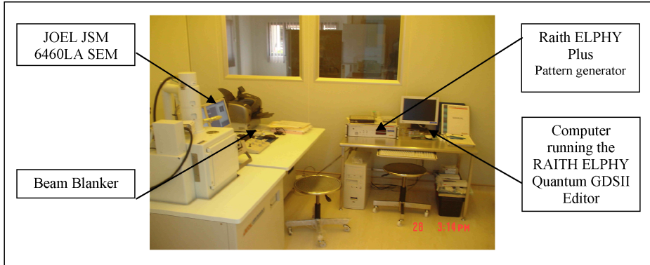
FIGURE 3. The EBL system at UniMAP's Microfabrication Cleanroom
