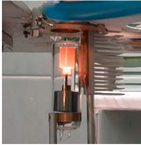
FIGURE 5. A Tantalum emitter situated in an Ar filled bulb under illumination from solar simulator
