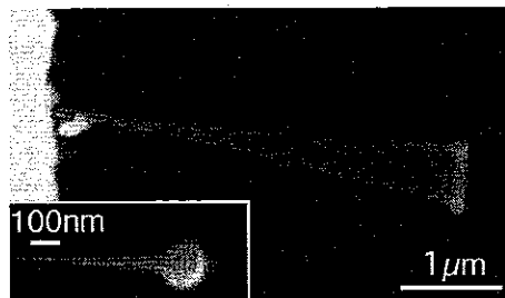
Fig. 1. SEM image of a carbon nanotube oscillator. The inset shows the deposit generated by an electron beam deposition process.
