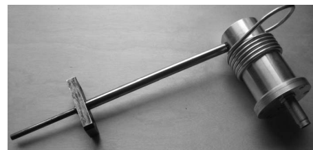
Fig. 14 DLR in-house design probe microphone
