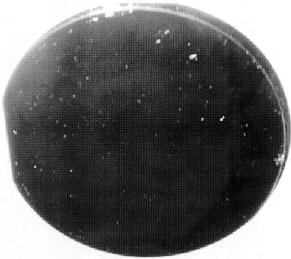
Fig. 5. Non-patterned bonded wafer stack. Bonding without massive air bubbles was done. Amount of non-bonded area was every time less than 5%. Non-bonded areas are seen as white dots.
