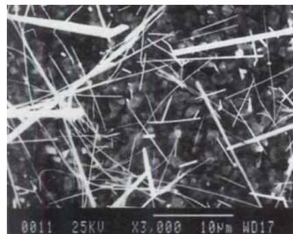
Fig. 5. SEM micrograph of a Cu-Se film on glass.
