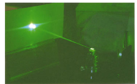
Fig. 2. A third-harmonic beam of green light was generated when an infrared light from an optical parametric oscillator passed through a 8-mm-long QPOS LiTaO 3 crystal.
