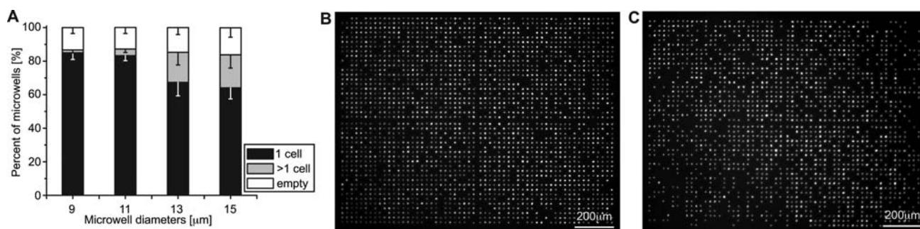
Fig. 3 Single-cell collection in the microchamber array. (A) Cell occupancy as a function of microwell diameters after the cell loading. (B) Loaded cells on the microwell array. 86.0% of 2552 wells (1/4 of a total area) contained single cells. (C) Captured cells in the microchamber array after the chamber-closing. 67.1% of 2552 chambers (1/4 of a total area) contained single cells. Repeated measurements (10 times) showed the single-cell occupancy of 65.4 \pm 7.8\% after the chamber-closing. (B) and (C) were visualized by the fluorescence microscopy of APC tagged cells.
