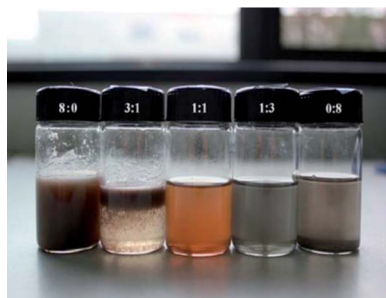
Fig. 2 The digital photos of the prepared inks with different solvent ratios of EG–EA = 8 : 0, 3 : 1, 1 : 1, 1 : 3 and 0 : 8.
