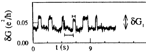
Figure 88. Time-dependent electrical resistivity of a submicron bismuth sample near 1 K where only tunnelling is possible. [Taken from Zimmerman et al. (1992), with kind permission of the American Institute of Physics.]
