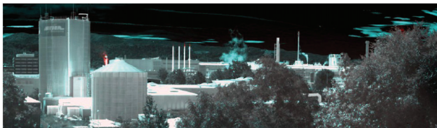
Figure 10. Bispectral infrared image of an industrial site taken with a 384 \times 288 dual-color InAs/GaSb SL camera. The two color channels 3\text{--}4\ \mu\text{m} and 4\text{--}5\ \mu\text{m} are represented by the complementary colors cyan and red, respectively (after [45]). (The color version of this figure is included in the online version of the journal.)
