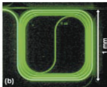
Figure 10 (online color at: www.lpr-journal.org) Top view image of a 4-cm-long spiral Er-doped waveguide wrapped up to fit in a chip area of \sim 1 \times 1 mm 2 . Green light owing to spontaneous emission on the ^2H_{11/2}/^4S_{3/2} \rightarrow ^4I_{15/2} transition is visible (Reprinted with permission from [230]. Copyright 2003, American Institute of Physics.).
