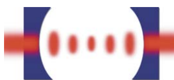
Figure 1 (online color at: www.lpr-journal.org ) Schematic representation of a Fabry-Perot cavity.
