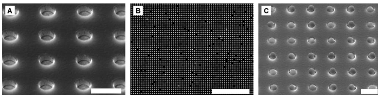
Fig. 4 Arrays of microwells and antibody-conjugated microbeads. (A) SEM image of a small portion of an array of \sim 0.5 \mu\text{m} wells at a 1.2 \mu\text{m} pitch etched in a silicon dioxide film that was deposited on a gold-coated wafer. (B) Raw fluorescence image of a small portion of an assembled array of 0.4 \mu\text{m} antibody-conjugated beads at a 1.2 \mu\text{m} pitch. (C) SEM image of a small portion of an assembled array of 0.4 \mu\text{m} antibody-conjugated beads at a 1.2 \mu\text{m} pitch. The scale bars in (A) and (C) are 1 \mu\text{m} . The scale bar in (B) is 24 \mu\text{m} .
