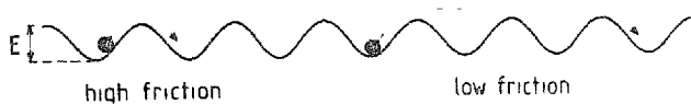
Fig. 10 Adsorbate diffusion on a corrugated one dimensional potential energy surface. For large friction \eta the adsorbate motion is strongly damped and only jumps between nearest neighbour potential wells occur. For small friction, once excited over the barrier, the adsorbate propagates for many lattice spacings before finally falling down in a well.
