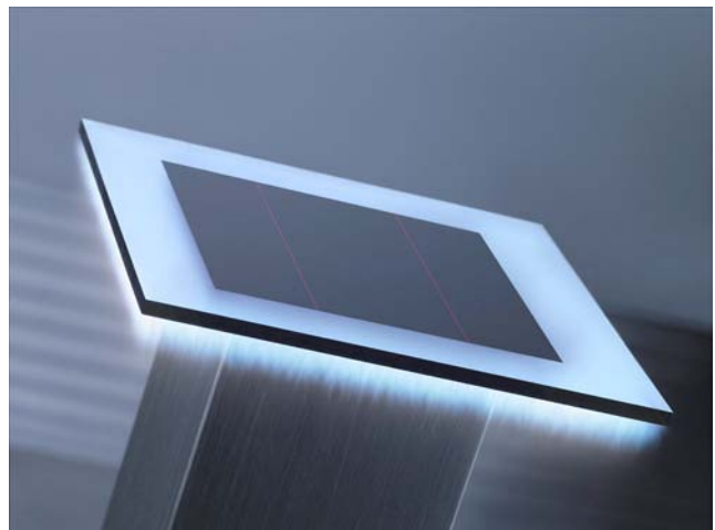
Figure 7 Thin film solar cell showing edge deletion conducted with the TRUMPF TruMicro 7050 laser
