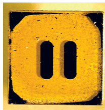
Figure 4.2 Deposited lateral contacts on CVD Diamond.
