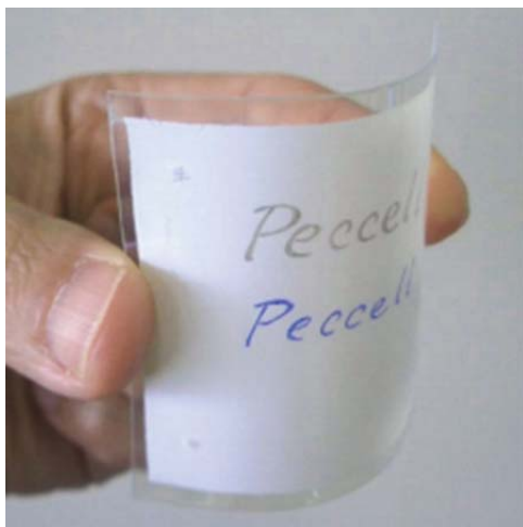
Figure 12. A photo of \text{TiO}_2 film coated on ITO/PEN, showing good film uniformity and good adhesion to the substrate. 33
