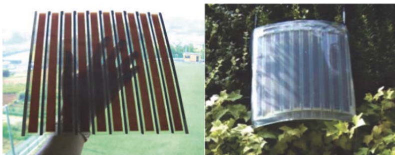
Figure 14. Flexible DSSC module based on \text{TiO}_2 film prepared by electrophoretic deposition. 36
