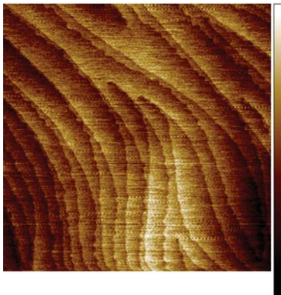
Fig. 4.7 AFM image of GaN film on Si substrate achieved by MMELOG with a 100 nm AlN buffer layer RMS = 0.148 nm ( 2\ \mu\text{m} \times 2\ \mu\text{m} scanning area); the thickness of GaN film is 3.2\ \mu\text{m}
