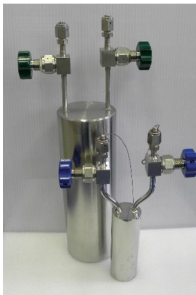
Figure 12.7 Standard bubblers for MO. Large one (100 mm in diameter) may contain 1.5–2 kg of TMGa. Small one (50 mm) – 150–200 g.
