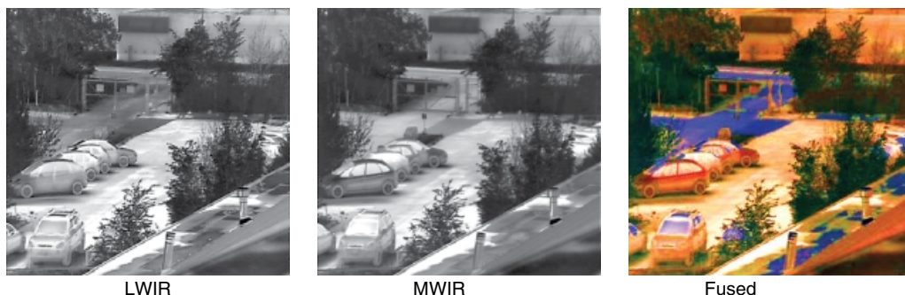
Figure 9.20 Imaging from CONDOR bispectral detector (F2, 4 ms/0.4 ms integration time). Source: Courtesy Leonardo MW Ltd.
