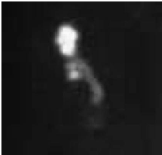
Fig. 3.2.32 Four-segmented cladding polymer fiber becomes few-moded.
