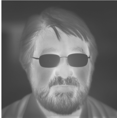
FIGURE 37.27 This image was taken by the R-QWIP FPA with 1024 \times 1024 pixels.
