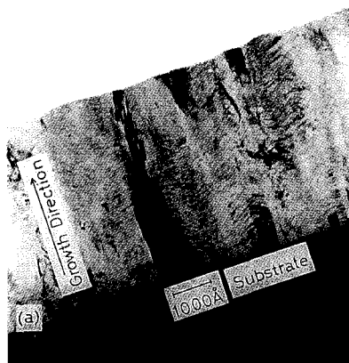
Fig. 49. Transmission electron micrograph of a cross-section of a MSD-prepared \text{ZnS:Mn} thin film (Ref. 179)
