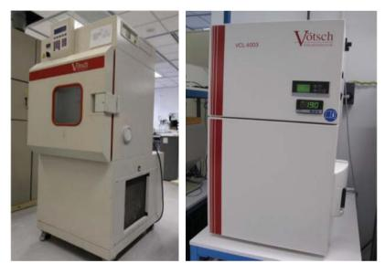
Figure 6.4 Typical thermal cycling chamber (left) and humidity chamber (right).
