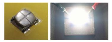
Figure 3.72 Singulated package assembled on a PCB.
