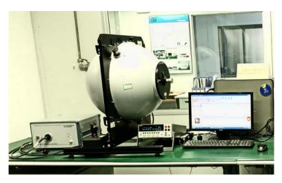
Figure 5.13 Typical integrating sphere system including a spectrometer (Instrument System CAS-140CT).
