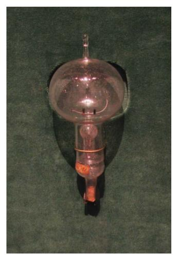
Figure 1.7 Edison's first successful lightbulb demonstrated to the public. Source: https://commons .wikimedia.org/wiki/File:Edison Carbon Bulb.jpg#/media/File:Edison Carbon Bulb.jpg.
