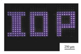
**Figure 7.8** Representative micro-displays programmed onto the flip-chip blue micro-LED array [30]. Source: Gong, Z., Gu, E., Jin, S.R. et al. Efficient flip-chip InGaN micro-pixellated light-emitting diode arrays: promising candidates for micro-displays and colour conversion. *Journal of Physics D Applied Physics*, 2008, 41(9): 094002.
