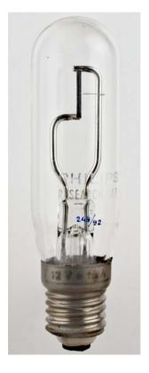
certain current, its resistance can be monitored. The electrical resistivity of tungsten is temperature dependent. As a result, the temperature can be calculated from a precalibrated temperature-resistance curve. Once the temperature is achieved, the radiation intensity and spectrum can be easily calculated according to Planck's law.
