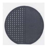
Figure 3.68 Through silicon slots by DRIE.
