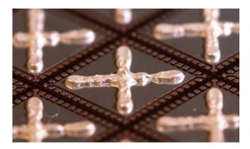
Figure 2.10 Die attach adhesive dispensing pattern. Source: Henkel.
