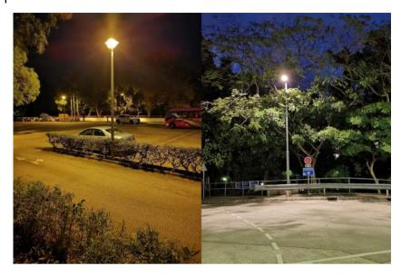
Figure 5.8 Comparison of the color presented by high pressure sodium lamp (on the left) and LED (on the right) on a cement road surface.
