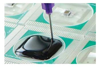
Figure 4.29 Glob top dispensing [41]. Source: Source: NICHE-TECH. 2019. http://www .nichetechcorp.com/ (cited date 3 September 2020).
