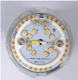
Figure 4.23 Board level assembly with multiple LED components.
