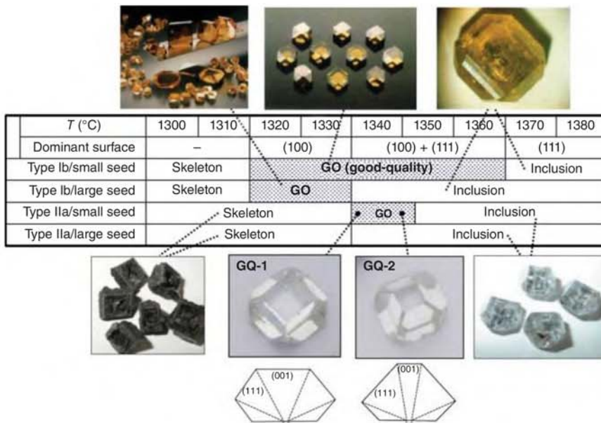
Figure 20.5 Cubo-octahedral-shaped diamond crystals grown by the temperature gradient method at different temperatures. Substitutional nitrogen ( \approx 100 ppm) causes the yellow color of the Ib-type crystals in the upper row. In the type IIa crystals in the lower row, the nitrogen concentration is < 0.1 ppm. Source: Reprinted with permission from Sumiya and Tamasaku [28]. © 2012 The Japan Society of Applied Physics.
