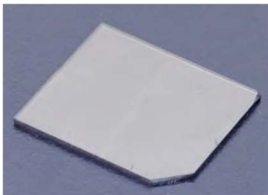
Figure 21.4 Tiled clone with 20-mm edge, where four single-crystal diamond substrates with 10-mm edges were connected with each other.
