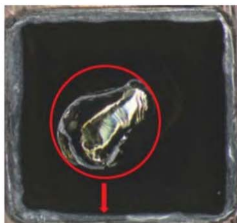
Figure 14.19 Shell-like crack at backside of the chip after doing 2570 pulses with 220 A/10 ms at a 20 A/1200 V SiC MPS diode.
