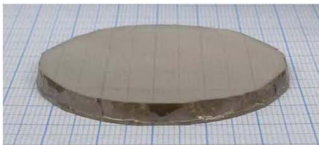
Figure 18.10 Am-GaN crystal grown in one crystallization run: 6-mm-thick and with a 2.1-in. diameter; grid 1 mm.
