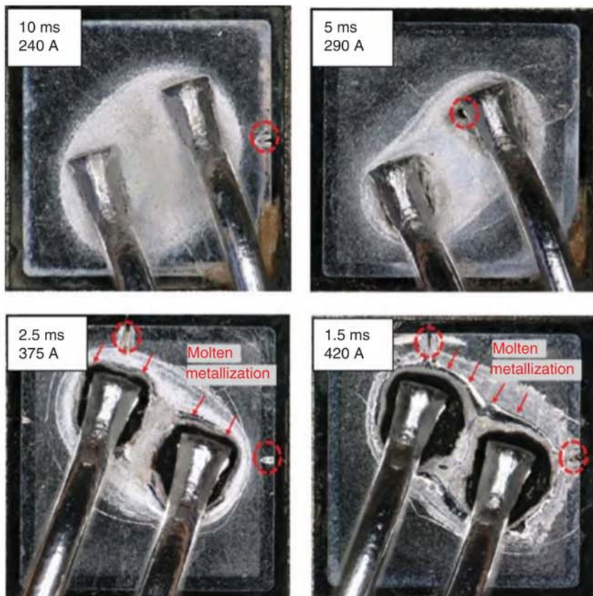
Figure 14.14 Failure pictures after single-event destructive surge-current pulses with a 1200 V/20 A SiC MPS diode.
