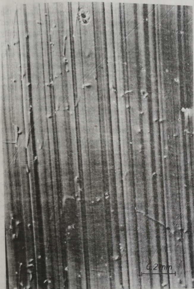
Fig. 13. Photomicrograph (interference contrast) of n-GaAs after photo-etching with an \text{H}_2\text{O}_2/\text{H}_2\text{SO}_4 solution for revealing crystal defects [18] .
