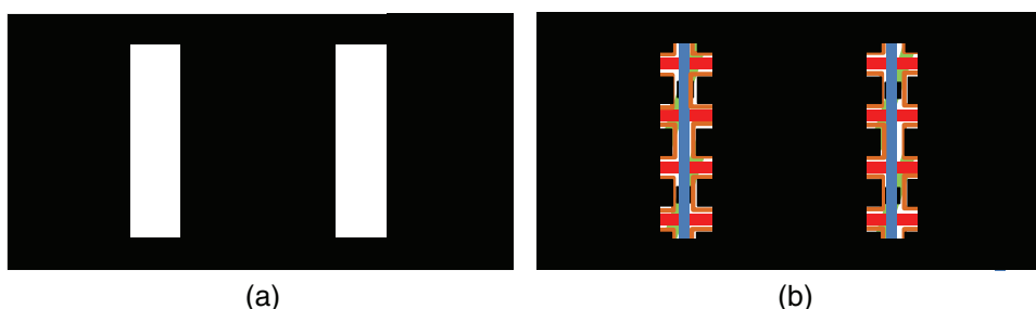
Figure 1.44 (a) SiN slot mask and (b) slot mask overlaps with previous layers.
