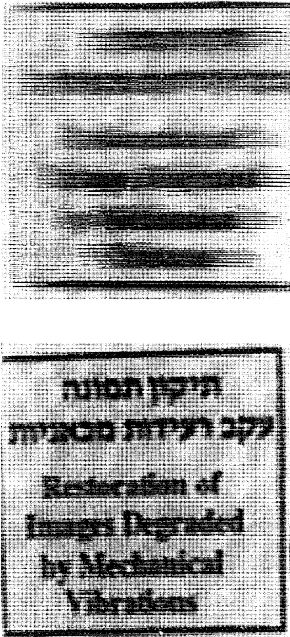
Fig. 18.1 Low vibration frequency (21-pixel linear motion blur extent) degraded and restored images (after [18.3]). Width of numbers is about 5 pixels. In the restoration process, \gamma = 0.2667 . (The English is a translation of the Hebrew.)
