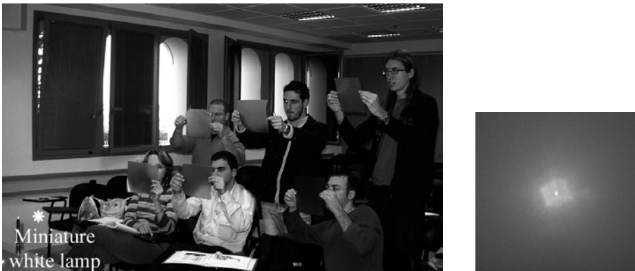
Figure 11.11 Viewing a compound computer-generated hologram using as an illumination source a miniature white-light lamp (left) and one of the views reconstructed from the hologram (right).
