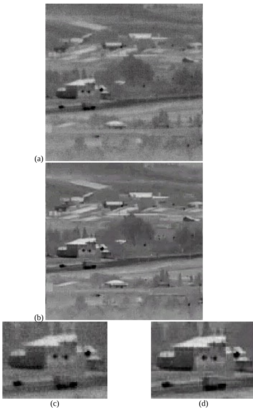
Figure 11.7 Examples of frames of (a) initial and (b) restored thermal real-life video sequence, and (c) and (d) corresponding magnified fragments of the images. Note enhanced sharpness of the restored image.
