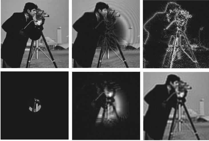
Figure 1.1 Results of the cameraman image filtering in fractional FT domains for \varphi = 0, 3\pi/8, \pi/2 (from left to right). The upper (lower) row corresponds to the filtering with H (L) mask, respectively.
