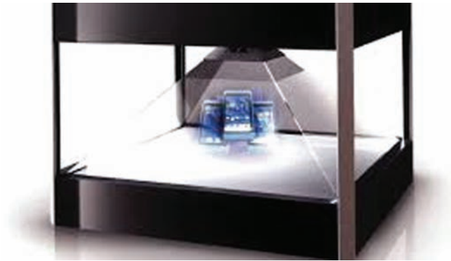
Figure 11.73 Example of the Pepper's ghost image produced by the Dreamoc™ display. In this case, the three display devices are embedded in the top of the device and project down toward the angled glass viewing "surface." © Realfiction.
