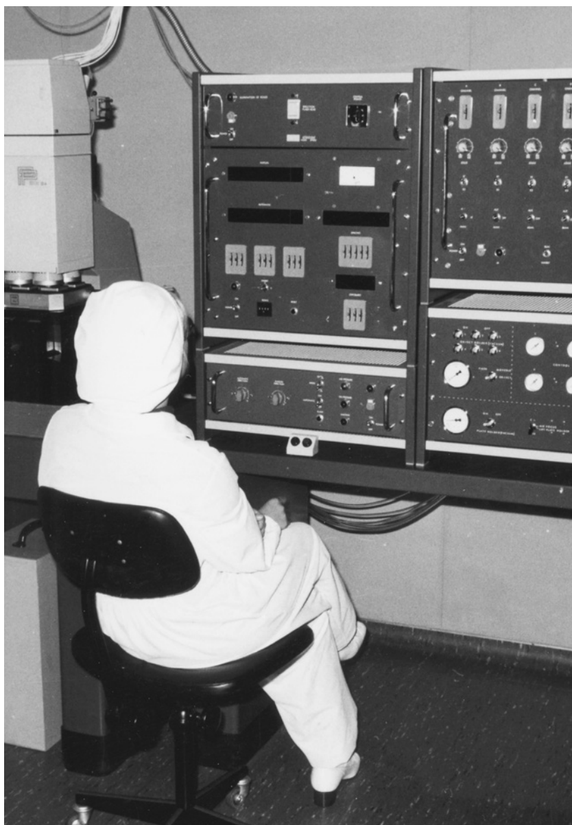
Philips' step-and-repeat camera (left) with operator. The dark cabinets on the right house all the control electronics, which were designed and built by Philips Elcoma in Nijmegen.
