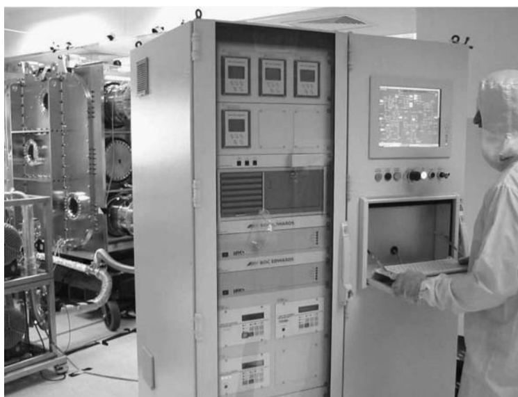
Figure 9.41 Vacuum control system interface.
