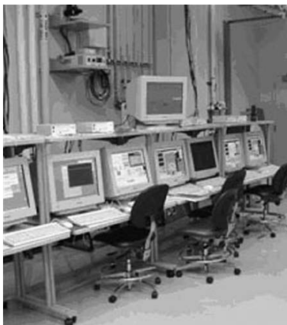
Figure 2.8 Control console for the ETS with graphic displays to control the wafer exposure and monitor the status of the LPP source, condenser, and PO flux systems. (Reprinted with permission from Intel.)
