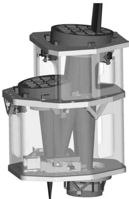
Figure 6A.2 Projection optics box from the ETS. All four mirrors are coated with normal-incidence ML coatings.
