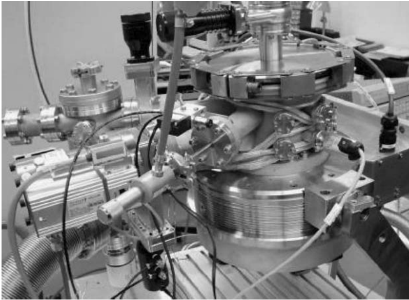
Figure 9.25 EUV Xe DPP source during brightness testing.
