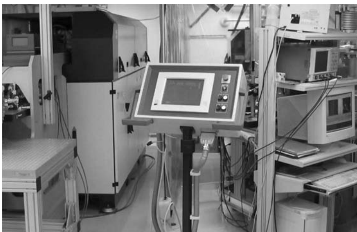
Figure 19.6 Photograph of the 1.2-kW laser (left-hand side, in the background) in XTREME technologies' high-power LPP EUV laboratory.
