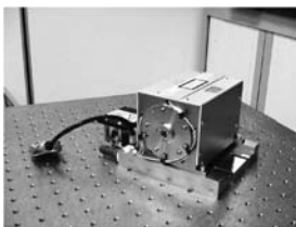
Figure 21.19 Diode pumping structure.
