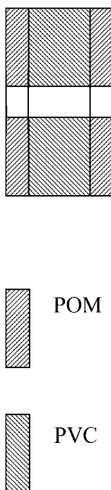
Figure 18.5 Construction of a typical PVC capillary. The end caps are typically 5 mm in length, while the PVC section in the middle has a length between 20 and 30 mm.
