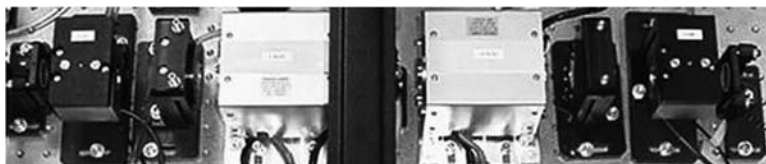
Figure 21.18 Twin-laser-head cavity design to increase beam quality and output power of SHINE.
