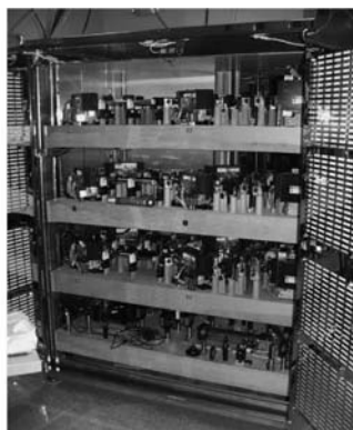
Three 1500-W laser modules in enclosure
