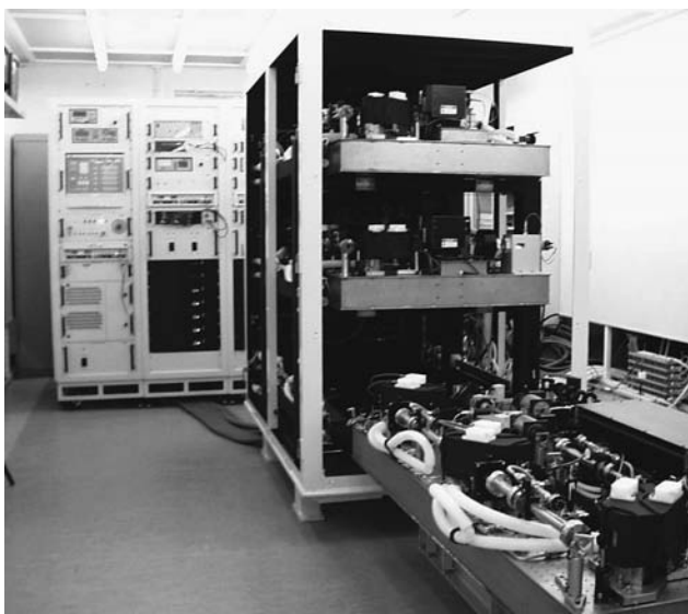
Figure 24.5 High-power Nd:YAG laser with two chains installed and one chain on loading rails. Controller can be seen in the background.
