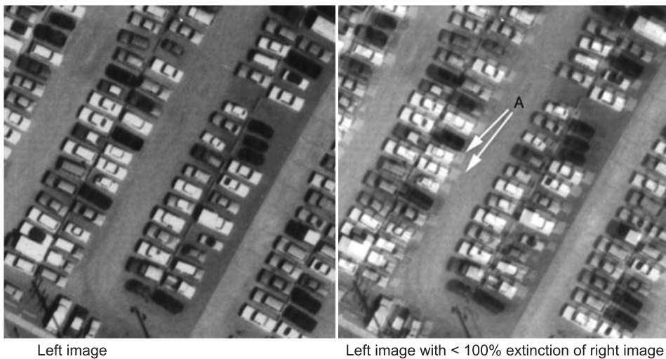
Figure 9.1 Effect of less than complete stereo extinction.
