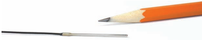
Figure 11.26 Photograph of a fiber Bragg grating temperature sensor (photo courtesy of Micron Optics Inc.).
