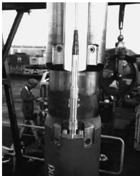
Figure 12.13 Fiber optic pressure gauge installation (reprinted from Ref. 3 with permission, © 2003 Elsevier).
