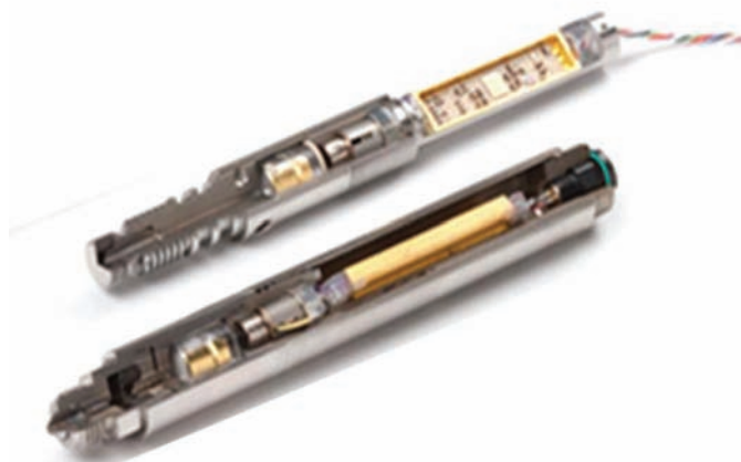
Figure 12.1 Quartz resonant gauge courtesy of Quartzdyne Inc.
