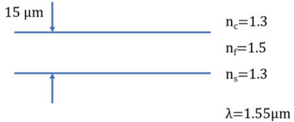
Fig. 3.16 A slab waveguide
