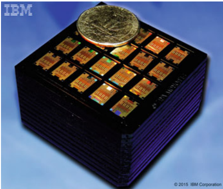
Fig. 1.1 IBM demonstrated its first fully integrated wavelength multiplexed silicon photonics chip. Source https://arstechnica.com/informationtechnology/2015/05/ibmdemos-first-fully-integratedmonolithic-siliconphotonics-chip/
