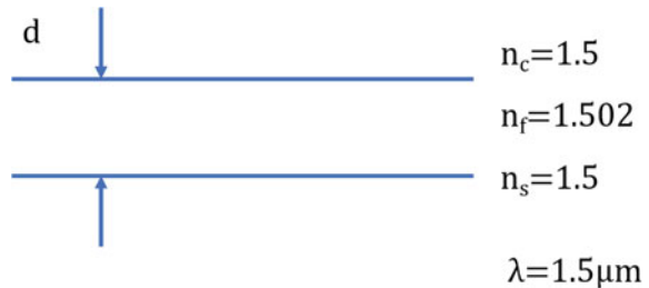
Fig. 3.17 A symmetric slab waveguide
