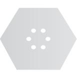
high losses due to leakage into the cladding, whereas the fundamental mode exhibits only very weak leakage. Mode areas well above  $1000\ \mu m^2$  are possible without excessive bend sensitivity. Further improved versions can contain an additional ring of air holes around the inner ring.
