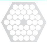
confined in the silica, even if the core is made rather small. For the calculation of the modes, it is essential to use a full vectorial model, as a scalar approximation (considering only the electric and magnetic field in a single direction) fails. The guiding properties of such fibers are not too different from those of a cylindrical piece of silica with a diameter approximating that of the core structure.
