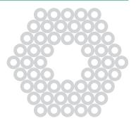
that the amplitude decays exponentially. As a result, light in the core structure cannot escape into the cladding, even though its intensity distribution may somewhat penetrate the cladding. The core can even be hollow, as in the example shown with seven missing tubes.
