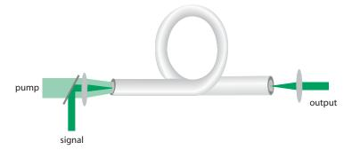
As alternative solutions, various types of fiber-based pump couplers allow one to avoid the disadvantages of free-space optics such as alignment issues, risk of contamination with dust, etc.
