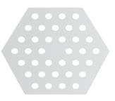
age refractive index due to the air holes. The larger phase delay in the center can compensate the natural tendency of light to diverge, and thus stabilizes one or several guided modes, depending on the hole size and spacing, and also on the wavelength.
