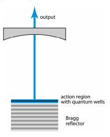
is completed with an external mirror and may contain additional optical elements. The external resonator allows for single transverse mode operation with larger active areas. With electrical pumping, ≈1 W of output power is possible in a diffraction-limited beam, with tens of watts possible from optical pumping, where it is easier to
