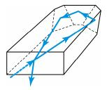
There are also monolithic ring resonators, such as the so-called **nonplanar ring oscillator** (NPRO), where the ring encompasses three points with total internal reflection and one reflection at the front face with a dielectric mirror coating. Pump
