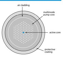
achieved with tiny air holes. Such fibers are called **photonic crystal fibers**.
