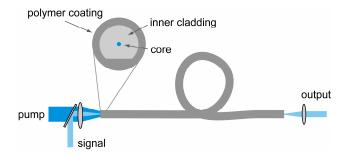
The figure shows a double-clad fiber amplifier. A laser could be formed by inserting two plane laser mirrors just outside the two lenses. However, high-power devices are more often made as "master oscillator power amplifiers," consisting of a seed laser and a power amplifier.
