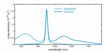
For example, the figure shows effective absorption and emission cross sections of ytterbium (Yb³+) ions in germanosilicate glass, as used in the cores of ytterbium-doped fibers.
