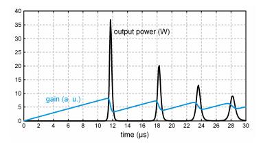
Gain switching can also be applied to optically pumped lasers (e.g., solid-state bulk lasers) by applying optical pump pulses from a Q-switched laser or from a diode laser in quasi-continuous-wave operation. The figure above shows a Nd:YAG laser simulation with a constant pump power turned on at t=0. If the pump power were applied for only 15  $\mu$ s, for example, only the first spike would be emitted, with a duration of only 0.35  $\mu$ s.
