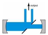
Another type of resonator uses a **scraper mirror** that sends some of the circulating light to the output. Variations of that scheme are applied to certain slab lasers, where the scraping is done on one side only.
