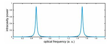
The figure shows the power in a resonator when the optical frequency is scanned through two subsequent axial resonances, and the profile of the input beam matches that of the fundamental modes. The full width at half maximum of such resonances is called the resonator bandwidth. It is proportional to the corresponding mode's rate of power losses (without incident light). A small bandwidth can result from low losses per round trip and/or from a long resonator length, such as long round-trip time.
