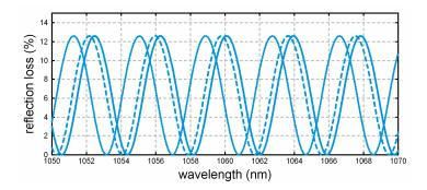
In principle, the interference effect is reduced by the tilt because it reduces the overlap of the counterpropagating beams, but this effect can be very small for thin etalons used in large-area laser beams.
