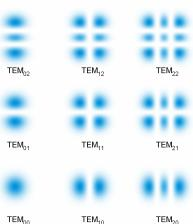
product of a Gaussian function and a Hermite polynomial. The lowest-order function of that type is Gaussian, while the intensity profiles of the higher-order modes are more complicated patterns (see the figure).
