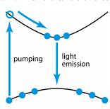
a somewhat shorter wavelength and involves the fast relaxation of carriers in both bands. Pumping is also possible with an electrical current sent through a p-n junction; carrier recombination occurs where the p and n materials meet.
