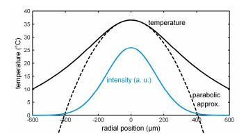
The temperature profile is often not quite parabolic, which means that the thermal lens has aberrations.
