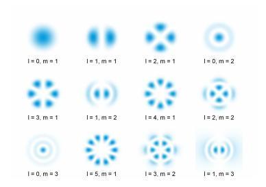
The figure shows the intensity profiles for every mode of an optical fiber (for a given design and wavelength). The lowest-order mode has a nearly Gaussian intensity profile, while the profiles of higher-order modes are more complicated. Generally, the number of waveguide modes increases with decreasing wavelength.
