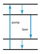
bypassing the laser transition itself, if the laser transition has a larger energy difference. (For longwavelength laser transitions, a laser crystal with low phonon energies is required to avoid this bypassing.)
