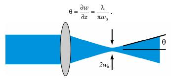
The equation shows that the **beam parameter product** (BPP), defined as the product of beam waist radius  $w_0$  and the divergence angle, is  $\lambda / \pi$  and thus independent of  $w_0$ . In fact, a Gaussian beam has the smallest possible (diffraction limited) BPP, which can be interpreted as the highest possible **beam quality** (see the next page).
