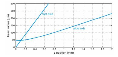
Beam collimation has to take care of the asymmetric beam profile; two cylindrical lenses are often used.
