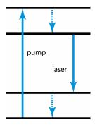
Laser gain with a much lower excitation level is possible in a four-level system, such as Nd:YAG. Here, the lower level of the laser transition is somewhat above the ground state, and a rapid (most often nonradiative) transfer from there to the ground state keeps the population of the lower laser level very small. Therefore, a moderate population in the third
