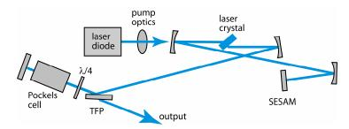
Design challenges can arise from the dispersion and Kerr nonlinearity introduced by the Pockels cell, which can affect the pulse formation process.
