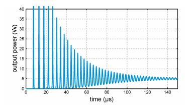
The essential dynamics of **spiking** and **relaxation oscillations** can be studied with a simple set of two coupled differential equations that describe the coupled evolution of optical power and laser gain. The following approximate formula is useful for determining the relaxation oscillation frequency:
