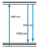
One benefit of quasi-three-level lasers is that they can have a rather low quantum defect (the difference between pump and laser photon energy) and thus a potentially high power efficiency. However, it is often not easy to realize this potential. Certainly, laser designs that are specifically adapted to such gain media are required.
