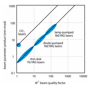
Even at high power levels, CO<sub>2</sub> lasers often reach nearly diffraction-limited beam quality. Due to the longer wavelength, the beam parameter product is larger than that of diffraction-limited solid-state lasers (e.g., thin-disk lasers), but it is still smaller than that of many solid-state lasers with nonideal beam quality. The figure above gives a rough indication of the typical parameter regions.
