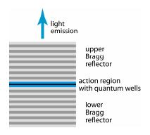
wafer surface. The laser resonator consists of a thin active region with one or several very thin (quantum well) amplifying layers sandwichedbetween distributed Bragg reflectors (DBRs). where one has a very high reflectivity and the other (the
