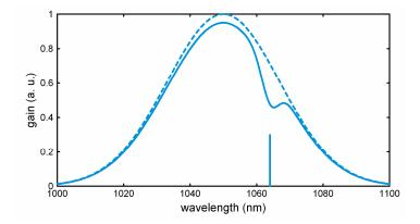
Obviously, saturation effects are significantly more complicated to calculate in the case of inhomogeneous saturation. They can have a significant impact on the operation of wavelength-tunable and single-frequency lasers
