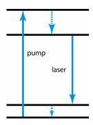
picoseconds.) As a consequence, the threshold pump power can be significantly increased, although not as strongly as in a true three-level system.
