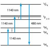
In principle, such processes are also possible in solid-state bulk lasers. However, they are normally more efficient in fiber lasers, where high pump intensity can be achieved over a long length of material. Good examples are thulium-doped blue lasers (see above) and praseodymiumdoped lasers with an emission of red, orange, green, or blue light.
