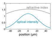
medium with a radially decreasing refractive index, as shown in the figure. The beam then experiences a focusing effect, which can exactly balance diffraction for certain beam profiles. The wavefronts then stay planar everywhere.
