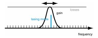
An adjustable optical filter may be introduced into the laser resonator, which has a pronounced loss minimum at some wavelength, forcing the laser to operate close to that wavelength. This is applied to many types of lasers. For example, a birefringent (Lyot) filter may be used within a Ti:sapphire laser or an external-cavity diode laser's diffraction grating.
