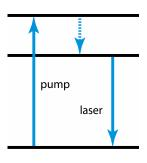
crystal) transfers atoms to an intermediate level, called the upper laser level. From that level down to the ground state, the laser transition with stimulated emission can occur. With sufficiently high pump intensity, population inversion for the laser transition can be reached as stimulated emission by the pump radiation is prevented by the transfer to the intermediate level. Also see p. 52 for quasi-three-level gain media.
