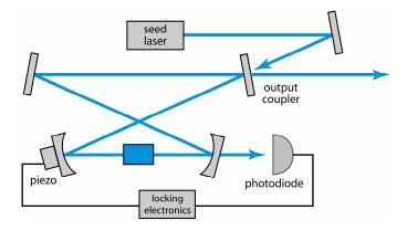
Here, a single-frequency signal from a low-power seed laser is injected into the high-power laser; this "slave" laser can be forced to operate on the same frequency, provided the injected optical frequency is sufficiently close to the resonance of the slave laser resonator. That condition is usually maintained with an automatic feedback loop acting on the slave resonator length.
