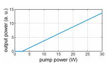
versus input power is called **slope efficiency**. The figure shows a case with a threshold power of 2.5 W and a slope efficiency of 50%.
