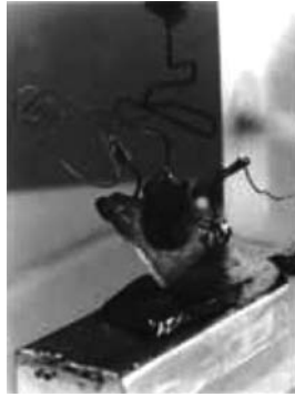
Figure 4.2 The first point-contact transistor. It was invented at Bell Laboratories on December 23, 1947. (Reprinted with permission from Alcatel-Lucent.)
