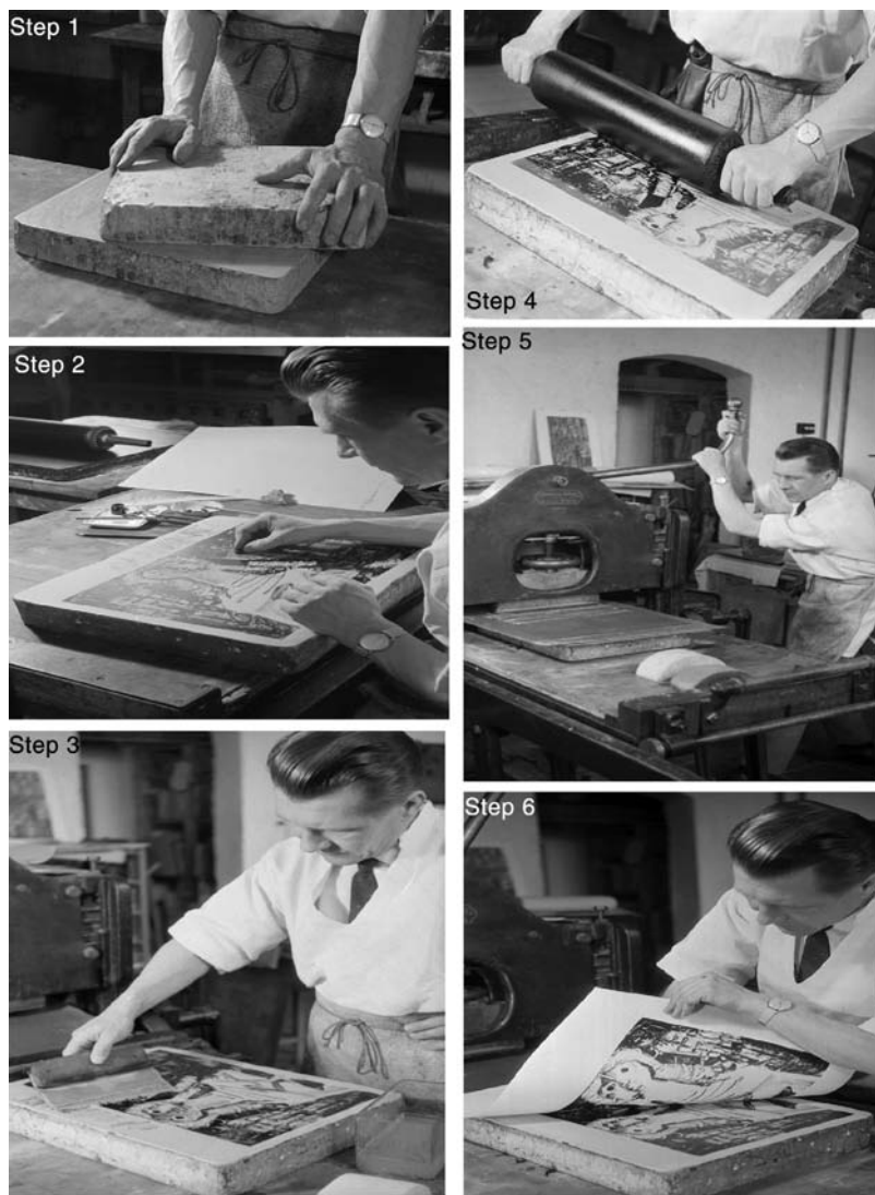
Figure 10.1 Stone lithographic process steps. Step 1: Polishing of the lithographic stone (today, polishing is done with a levigator). Step 2: The artist draws or paints on the lithographic stone with a greasy substance such as a litho crayon, paint, or pencil; the lithographic stone picks up this greasy substance and holds it. Step 3: Etching of the lithographic stone with a solution of gum arabic and nitric acid to prepare it for printing. The process of etching fixes the artist's image on the stone by making the dark areas very lipophilic and the light areas very hydrophilic. Following etching, the lithographic stone is moistened with water. The parts of the stone not protected by the greasy paint soak up the water. Step 4: Oil-based ink is rolled onto the stone. The greasy parts of the stone pick up the ink, while the wet parts do not. Step 5: A piece of paper is pressed onto the stone, and the ink transfers from the stone to the paper, effectively printing the image on the paper. Step 6: The printed paper is lifted off the lithographic stone, revealing the image. (Published with permission from the Deutsches Museum, Munich.)
