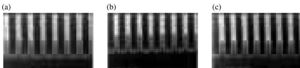
Figure 7.22 SEM images of 100-nm lines and spaces printed in a KRS-XE resist: (a) no PEB, (b) 80°C PEB, (c) 110°C PEB. (Reproduced with permission from IBM Corp. 344 )
