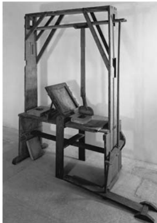
Figure 2.2 Wooden lithographic press constructed by Alois Senefelder and used in his invention of lithography. (Published with permission from the Deutsches Museum, Munich.)
