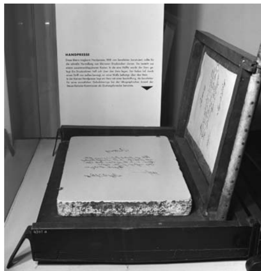
Figure 2.3 Lithographic stone and small hand press constructed by Alois Senefelder in 1818 and used for fast production of lithographic prints. Note the copy made from the handwritten note on the lithographic stone. (Published with permission from the Deutsches Museum, Munich.)
