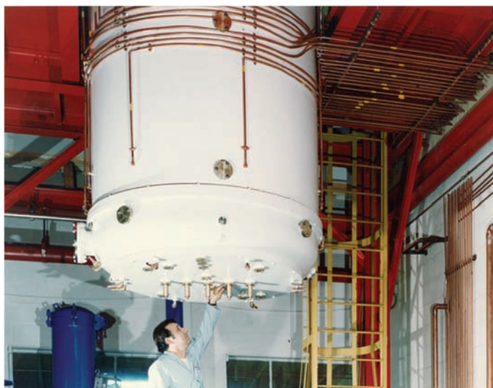
Figure 5.10 Installation of the first 52" production furnace.
