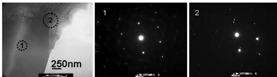
Figure 3.8 Princeton Scientific ZnS 40-k \times TEM and SAED of two regions. Region 1 is a bulk crystal region, and region 2 is on a thin twin. Both areas appear cubic.
