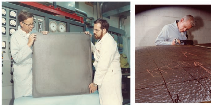
Figure 5.13 Inspection of large 34'' \times 34'' CVD ZnS plate.
