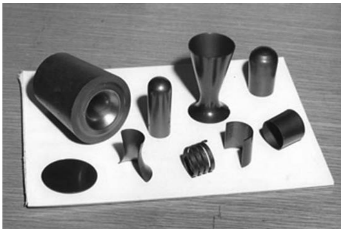
Figure 5.3 Various PG components, including rocket nozzles and nozzle inserts produced by the HTM Department.
