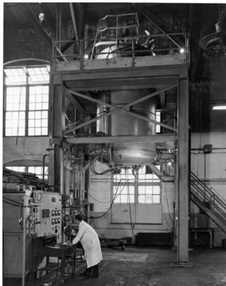
Figure 5.5 A large-scale, PG deposition reactor in Raytheon's HTM plant.
