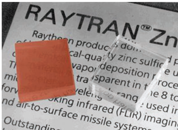
Figure 6.1 Standard CVD ZnS (left) and multispectral ZnS (right) produced commercially at Raytheon. The transparency of multispectral ZnS is apparent when viewing text through a ~3-mm-thick piece.
