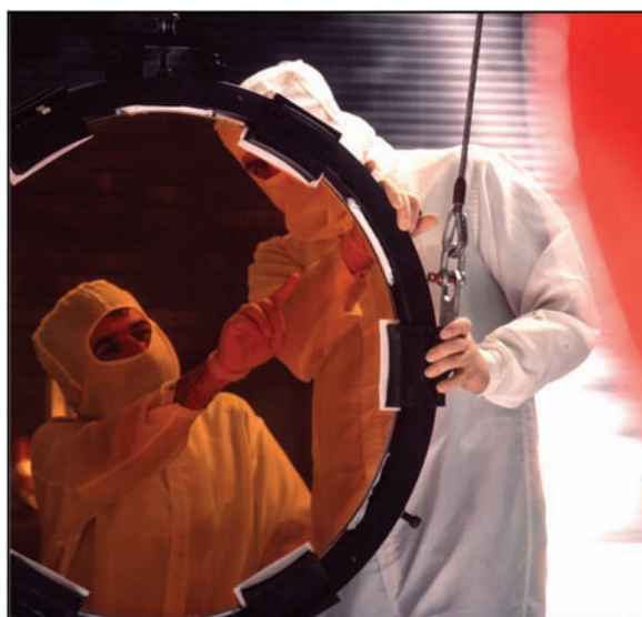
Figure 5.15 A large CVD ZnSe laser window produced at Raytheon, demonstrating the size and optical quality capability of the CVD process.
