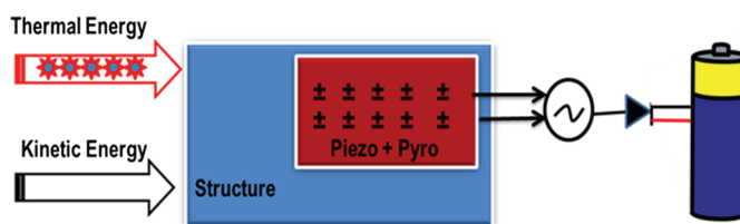
Figure 14 Concept and principle of a piezoelectric and pyroelectric mechanism.
