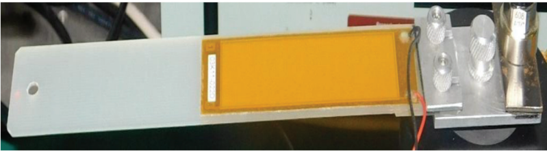
Figure 11 A photograph of a PZT cantilever clamped at one end.
