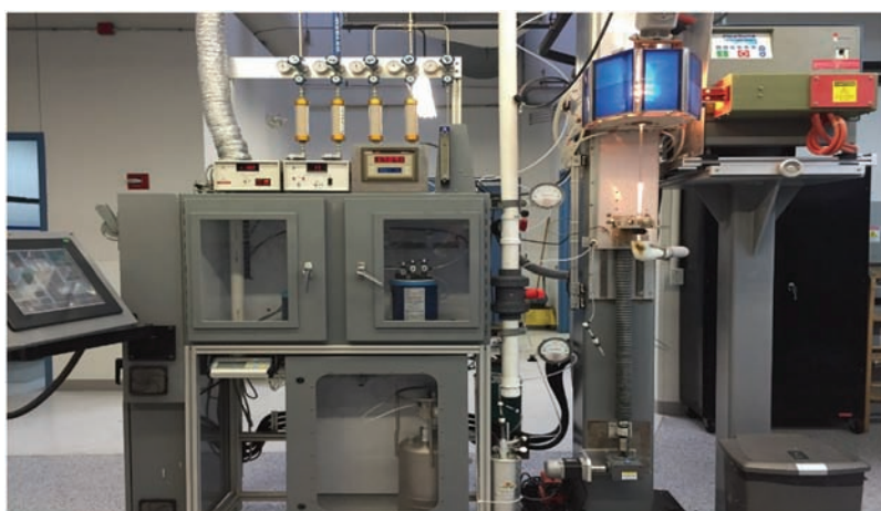
Figure 3.1 Creating the glass preform: a chemical vapor deposition preform tower.
