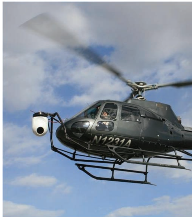
Figure 3.18 Ultra high-definition (UHD) cameras and high-speed gimbals require extremely precise stabilization and pointing in demanding environments. KVH UHD camera and gimbal customers require gyros with low noise, low drift, high bandwidth, and superior accuracy, and they have therefore selected KVH DSP-1750 or DSP-1760 FOGs to provide two or three axes of stabilization for their systems.
