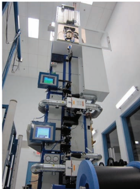
Figure 3.2 The fiber-drawing tower, which can produce up to 5 km of E•Core fiber from a single 1-m preform tube.
