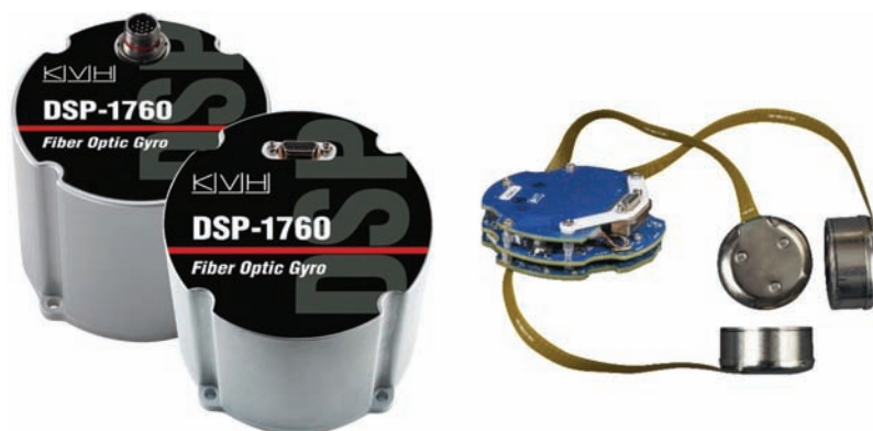
Figure 3.12 The KVH DSP-1760 FOG, which offers one-, two-, and three-axis configurations in both housed and unhoused variants for increased versatility.
