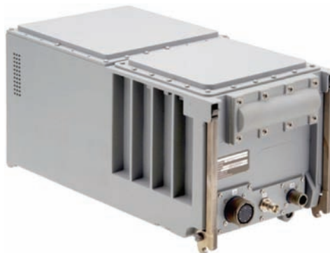
Figure 5.8 LN260 standard inertial navigator.
