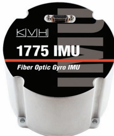
Figure 3.14 The KVH 1775 IMU is the highest-performing KVH FOG-based inertial system based on the E•Core ThinFiber technology. The 1775 IMU is available with \pm 10 -g or \pm 25 -g accelerometers.
