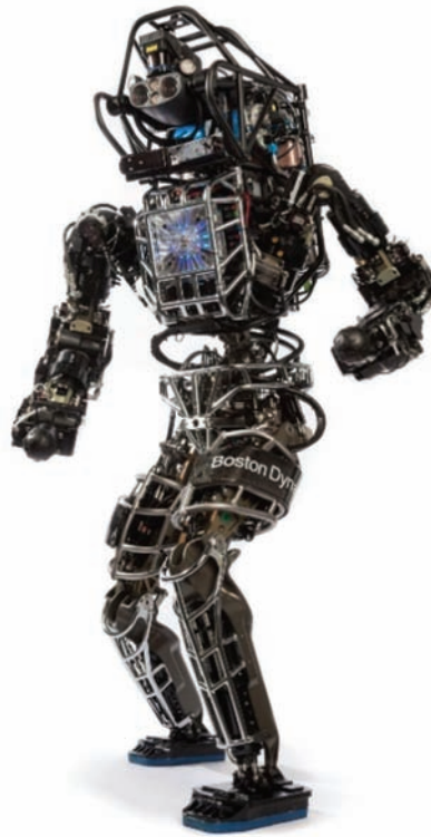
Figure 3.19 Eleven of the 23 robot finalists in the live hardware portion of the 2015 DARPA Robotics Challenge stayed on track thanks to the integration of a KVH FOG-based 1750 IMU within their systems. KVH IMUs were integrated into several of the entries, including the ATLAS robot platform by Boston Dynamics (shown here), as well as the eventual winner of the challenge.
