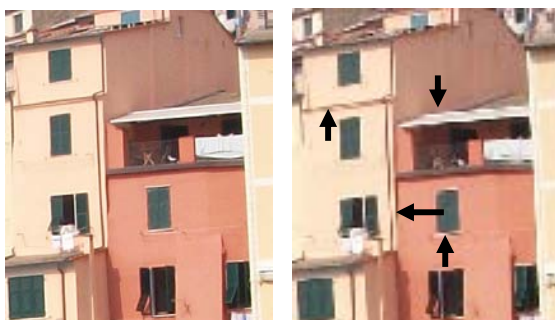
Figure 9-22. Original image (left) and image seen on the Windows XP desktop background scene (right). Each picture is 210×245 pixels (H×V). The arrows point to the most obvious sampling artifacts. Careful examination reveals numerous others.
