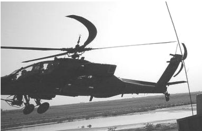
Figure 4-7. As object speed increases, the distortion produced by a rolling shutter becomes more apparent. Here it produces curved rotors. 23 Surprisingly, this ‘defect’ has created a new art form.
