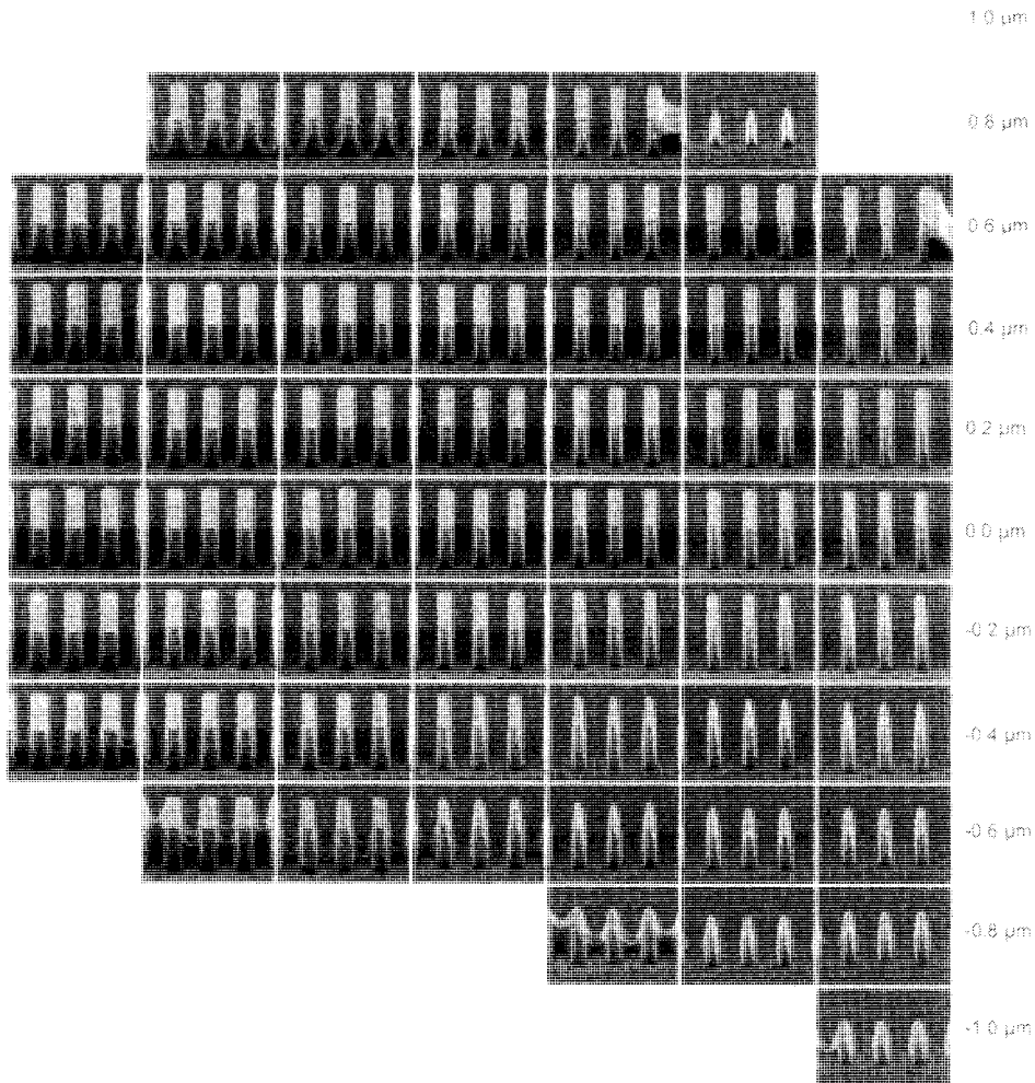
FIG. 1.31 Resist profiles for imaging at best focus and outside the depth of focus 20 .
