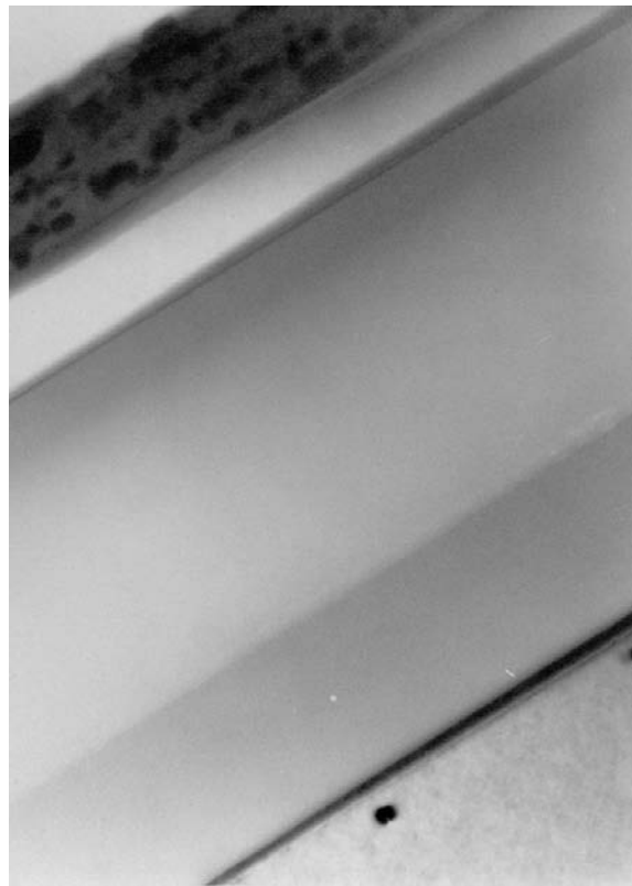
Figure 1.10. A scanning electron microscope image of a focused-ion-beam etched (FIBE) vertical cross section of a completed SonG wafer showing the various layers in the structure viewed at an angle of 60°. The 130-nm silicon layer and the GaAs substrate are clearly visible, as is the location of the bonding interface between the BPSG layer on the SIMOX wafer and the PECVD oxide on the GaAs wafer [59]. The top of the sample was coated with a layer of tungsten prior to FIBE processing; this layer is also visible. The FIBE cross section and photomicrograph were made by Dr. A. Stanishevsky and Prof. J. Melngailis of the Laboratory for Ion Beam Research and Application at the University of Maryland, College Park, MD.
