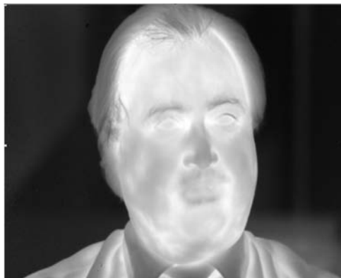
Figure 5.11. An image from a 640 \times 480 8.6-mm (long-wave IR) QWIP FPA thinned using the technique presented in this chapter. Target temperature differences as small as 20 mK can be resolved.
