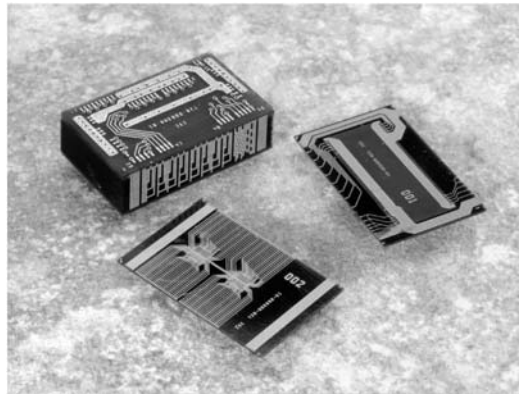
Figure 6.4. A molded integration example: the stack contains 16 layers of 64-Mb flash memory (layer shown on the right) and one layer of line drivers (layer shown on the left). Uppermost layer of the stack is a glass-epoxy based interface chip to the next packaging layer. The overall dimensions are 20 \times 12 \times 6 mm for a total capacity of 1Gb.
