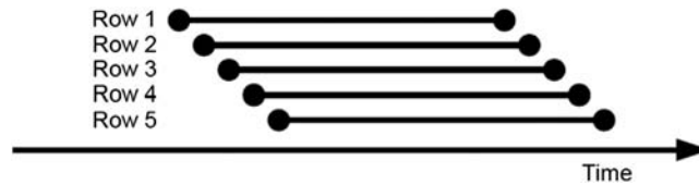
Figure 3.1 Line exposure window for five consecutive lines of a rolling-shutter sensor.
