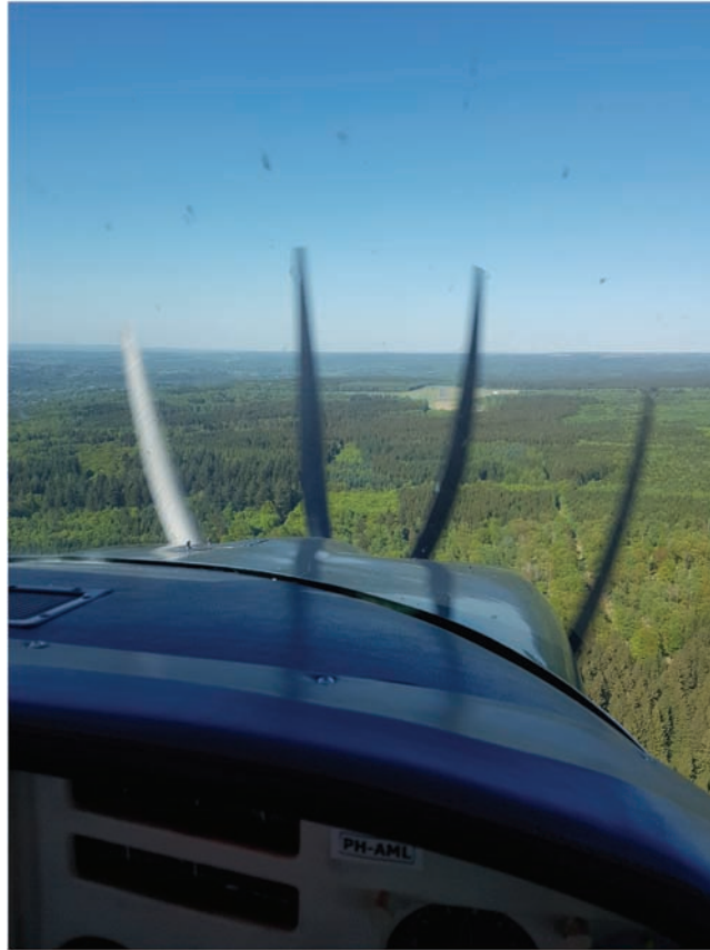
Figure 3.3 Plane propeller distorted by a rolling-shutter artifact.
