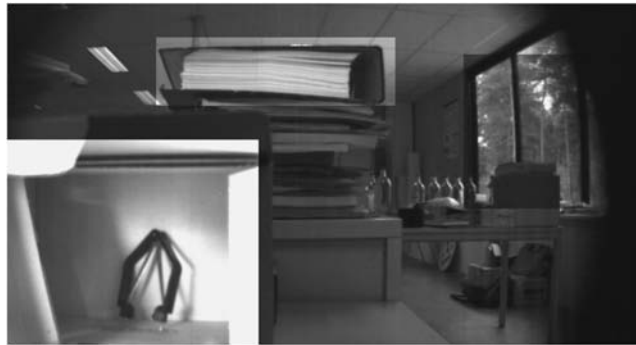
Figure 3.47 Use of multiple-exposure windows to extend the intrascene dynamic range (courtesy Melexis).
