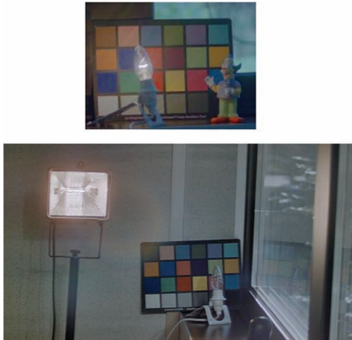
Figure 3.40 Images from a logarithmic photovoltaic sensor. Top: image of a color test chart with a lightbulb between the camera and the sensor; Bottom: image of a color test chart with a 330-W flood light (courtesy of NIT).
