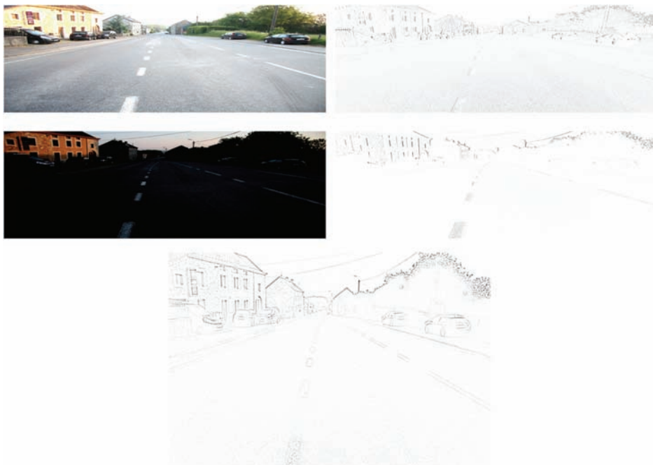
Figure 1.18 Road-marking-detection algorithm in an HDR scene without HDR imaging. Top left: even lines, long exposure. Top right: result of a horizontal edge detector on long-exposure lines. Middle left: odd lines, short exposure. Middle right: result of a horizontal edge detector on short-exposure lines. Bottom: combined and filtered binary edge image.
