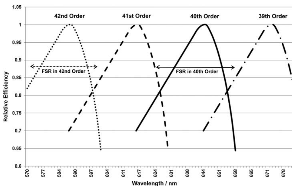
Figure 3.3 Efficiency of an Echelle grating at four subsequent orders.
