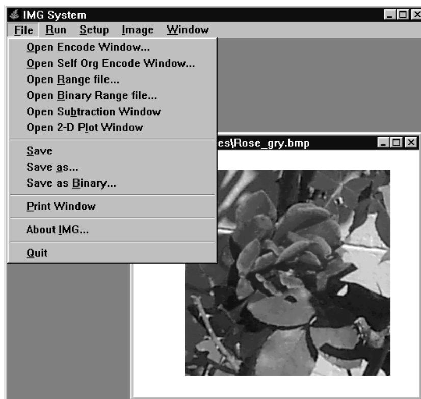
Fig. A.2.1 The IMG System for fractal image compression. The system can encode grayscale images using the fractal methods of Chapters 3 and 4 and can decode images stored as range files. The subtraction window provides error performance.
