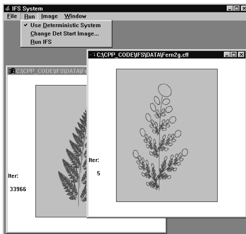
Fig. A.1.4 IFS window, showing a fern IFS generated with the random (right) and deterministic (left) algorithm. The starting image for the deterministic algorithm is a circle in this example.
