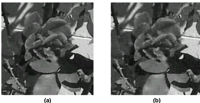
Fig. 6.6.1 Image compression of the “Rose” image using the D4 Daubechies wavelets. (a) 10% wavelet coefficients; average pixel error: 1.8929% (31.7549 dB PSNR). (b) 5% wavelet coefficients; average pixel error: 2.8264% (28.0999 dB PSNR).
