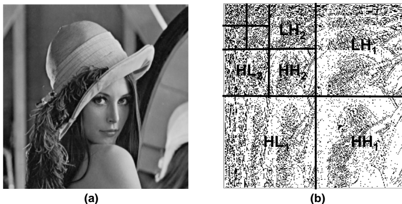
Fig. 7.2.3 The “Lena” image (a) and its wavelet transform (b). The image in (b) is formed by rendering the largest 50% of the Haar wavelet coefficients black and the remaining coefficients white. The wavelet subtree structure is superimposed here, with some of the highpass and lowpass operators identified. Note the similarity in corresponding blocks from one level to the next.
