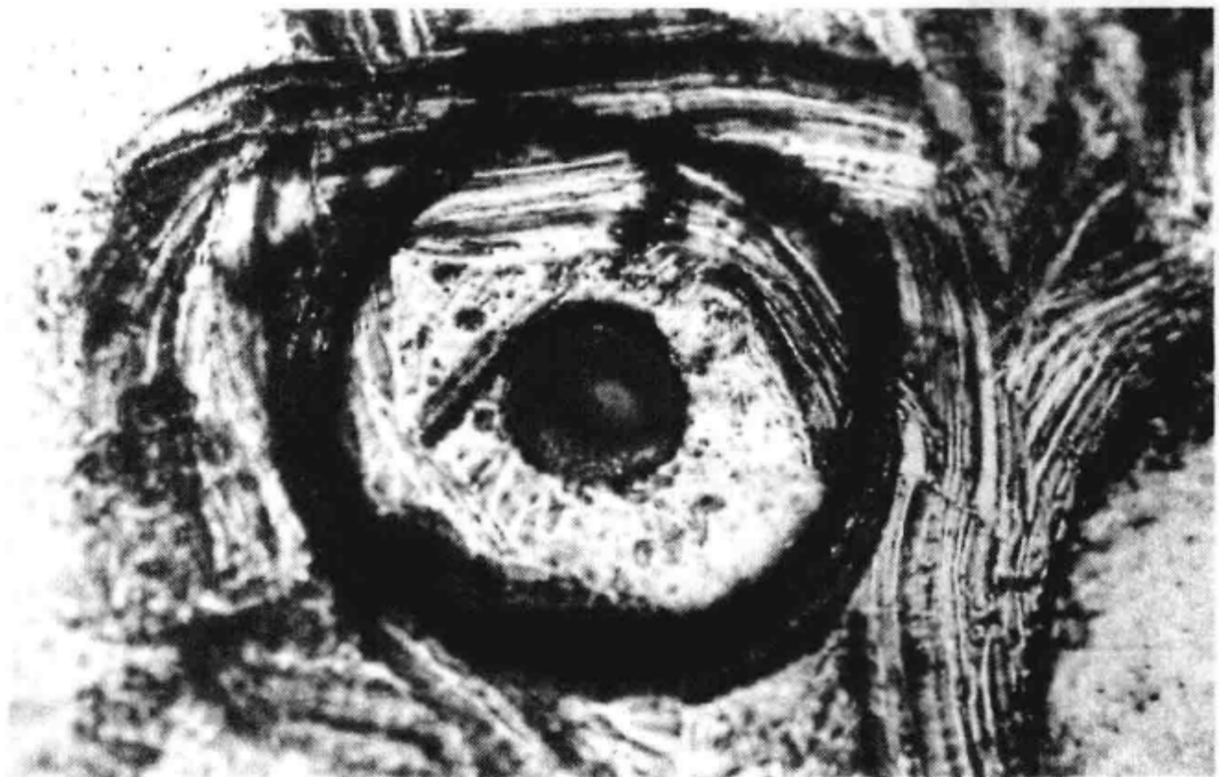
Figure C.19 A close-up (about 100×) of C.18, showing the pin broke off a piece of the glass fiber and moved it out of position.
